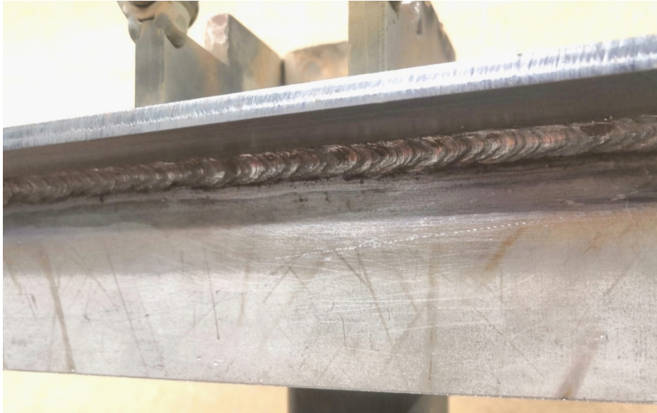
Figure 3. Pulsed MMA welded overhead fillet weld (welding position PD). Base material 5 mm structural steel S355 and filler material 3.2 mm basic electrode. Welding current 130 A and pulse frequency 1.5 Hz. The amount of spatter is minimal considering the welding application.
